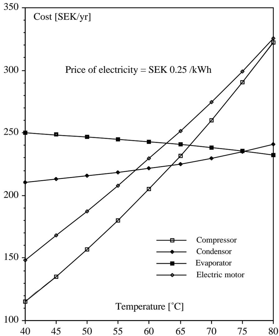
Fig. 8. Component costs as a function of the temperature of the produced heat.
