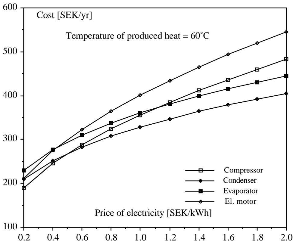
Fig. 6. Component costs as a function of the price of electricity when output heat is 60°C.
