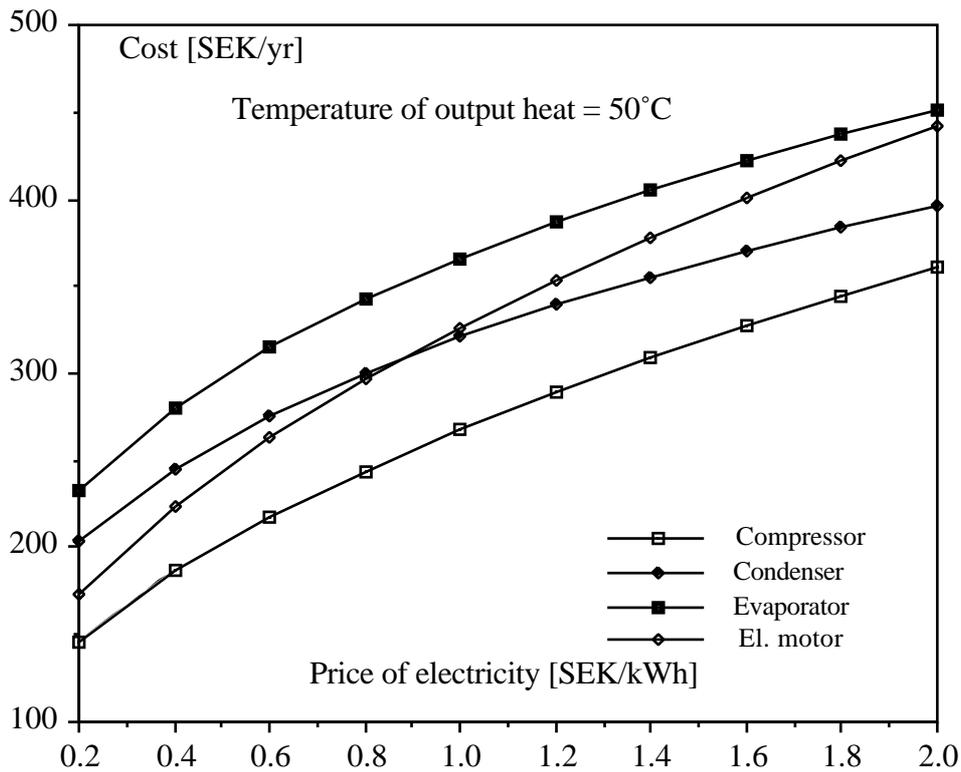
Fig. 5. Component costs as a function of the price of electricity when output heat is 50°C.
