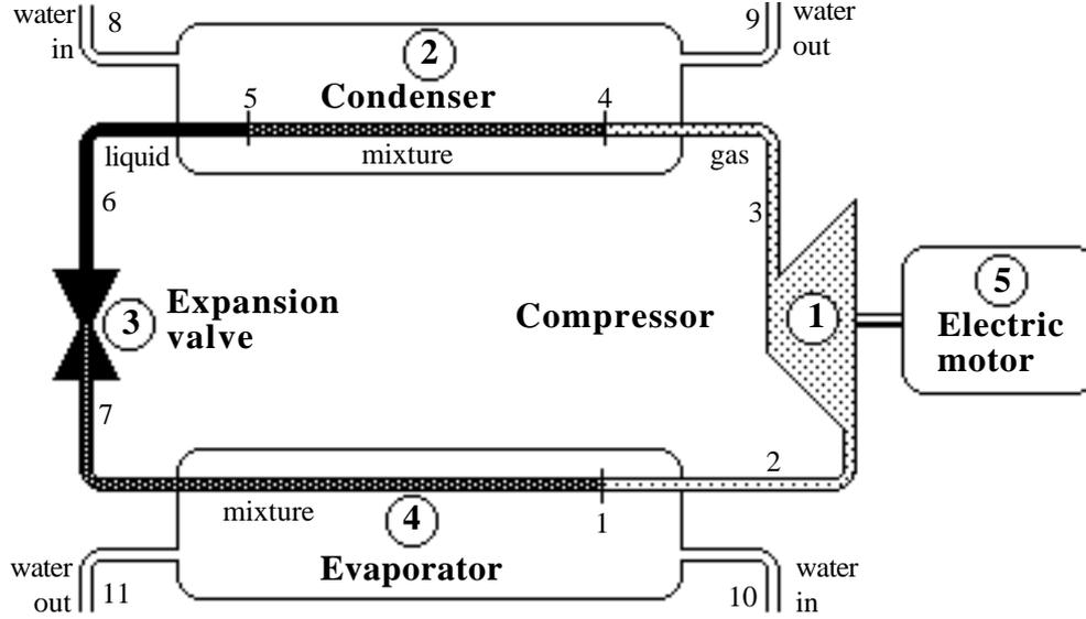
Fig. 2. Heat pump system with 5 components and 11 flows.
