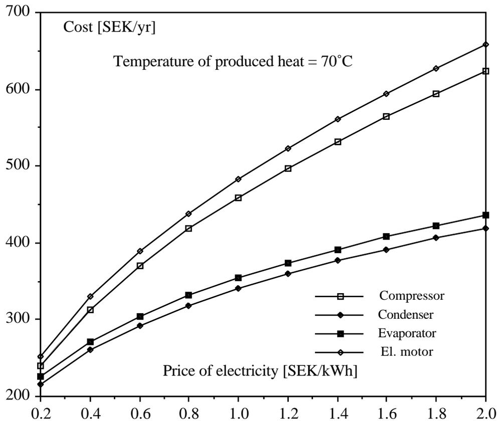
Fig. 7. Component costs as a function of the price of electricity when output heat is 70°C.
