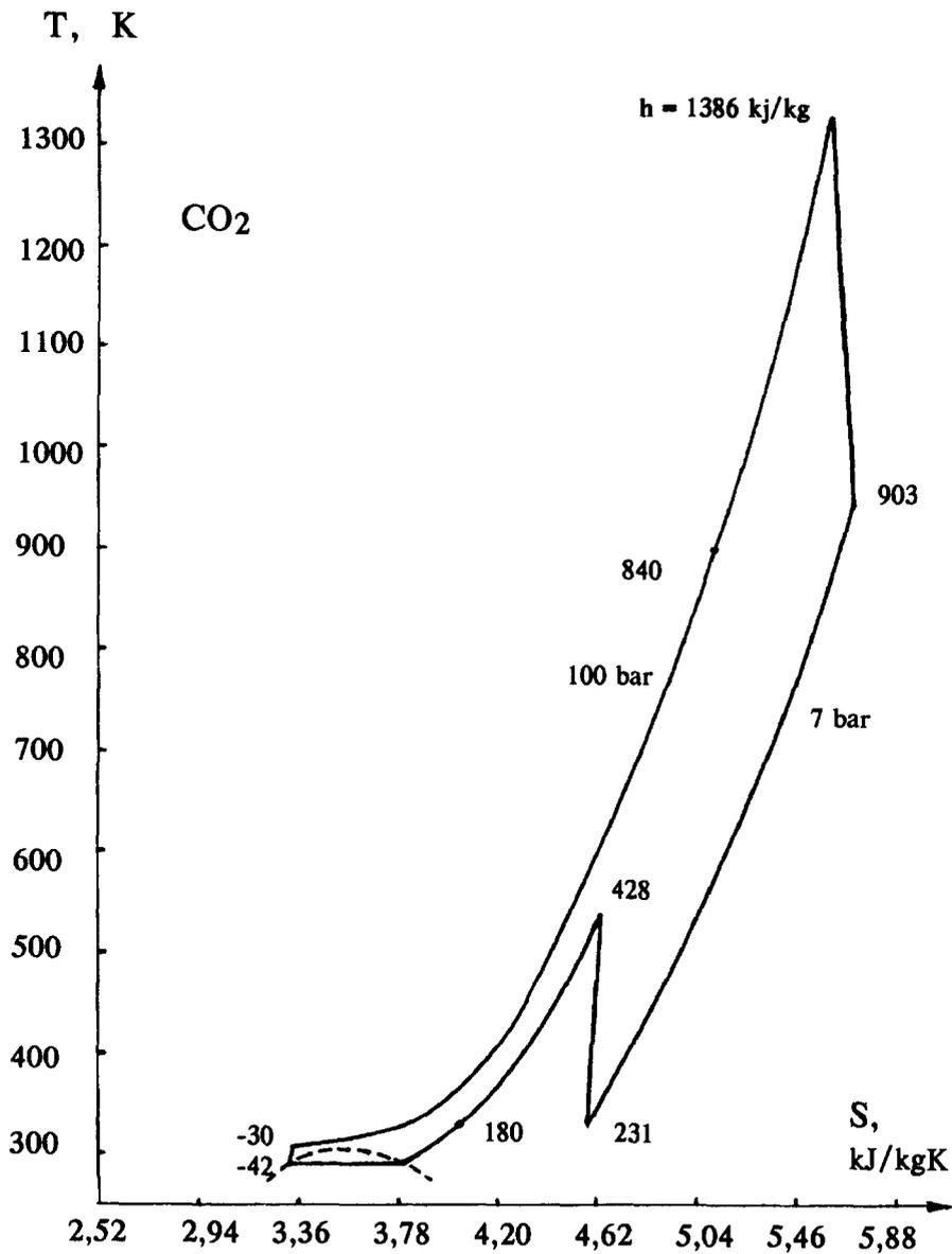
Fig.4. T-S diagram of the cycle with adiabatic compression and additional recuperators.
