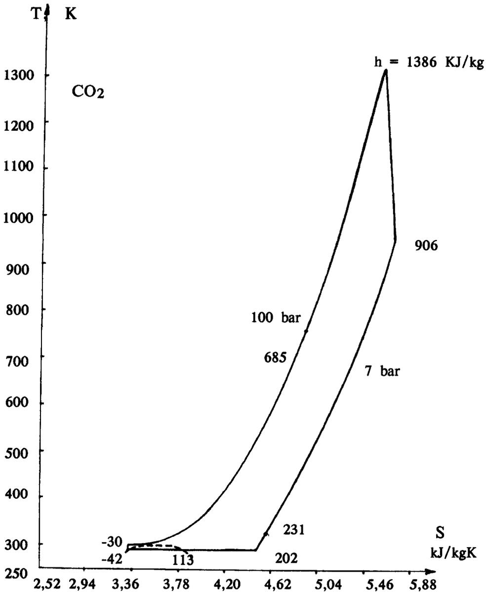
Fig.3. T-S diagram of the cycle with isothermal compression.
